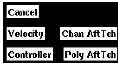
Figure 6: MIDI message assignment. Press one of the message types, or “Cancel” to return to the main screen.
