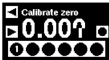
Figure 11: CV calibration screen. Press the round button to calibrate the zero point. Press the right arrow to proceed to the next step. Press the left arrow button to return to the previous step.
