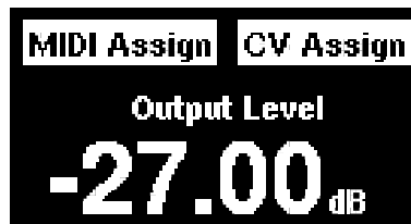
Figure 4: Parameter assignment buttons. Press “MIDI Assign” to assign this parameter to a MIDI message. Press “CV Assign” to assign the parameter to a CV input. Some parameters can be assigned to a gate input instead.
