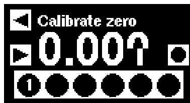
Figure 9: CV calibration screen. Press the round button to calibrate the zero point. Press the right arrow to proceed to the next step. Press the left arrow button to return to the previous step.
